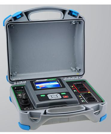
Digital Transformer Analyser (MI 3280) is a Multi-function, portable battery (Li-ion) powered test instrument with excellent IP protection: IP65 (case closed), IP54 (case open), intended for diagnosing of: turn ratio, phase deviation and excitation current of single and three phase transformers and winding resistance of single and three phase transformers.
