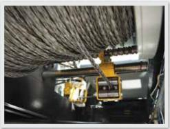
Anti-Twist Rope with Level Wind
